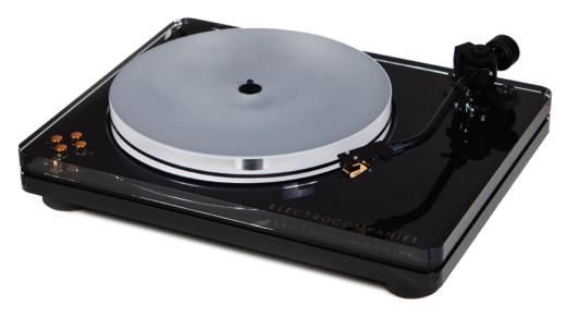
**CHASSIS:** The Electrocompaniet ECG-1 is a sandwich construction made out of three layers: acrylic and aluminum, benefiting from the internal dampening in the acrylic and the rigidity of the aluminum. This sandwich construction with its different materials increases the internal vibration dampening further, so the chassis will have no resonance problems.
