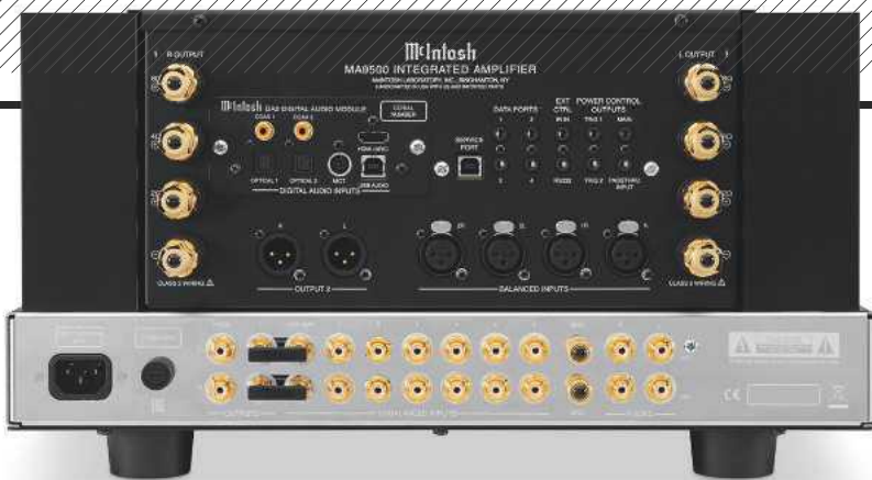
ABOVE: No fewer than eight line ins (six on RCAs, two balanced on XLRs) are joined by MM/MC, plus fixed (RCA) and variable (XLR) pre outs and 8, 4 and 2ohm speaker outputs. There are also four S/PDIF digital ins (two coax/optical) and a USB-B port
