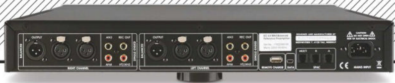
ABOVE: The preamp has two balanced (XLR) and three single-ended (RCA) ins, a line/rec out, and one balanced (XLR) output per side. BELOW: Power amp has switchable stereo/bridged mono inputs with daisy chain outs, all on XLRs. Two sets of 4mm speaker binding posts are offered per channel
